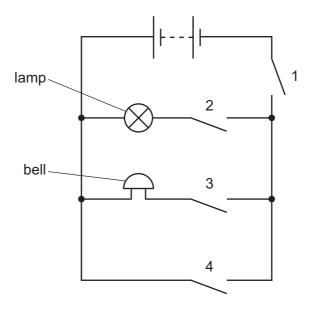
Which switches must be closed for the lamp to light and the bell to ring?
